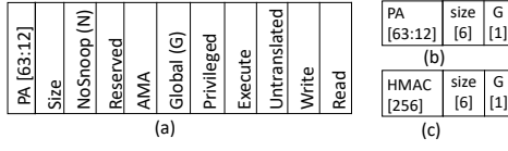
Figure 3. (a) Output of IOMMU() in eq. (1) with (PA, attr_{out}) . AMA: ATS Memory Attributes. (b) MOAT data structure to create AACs. (c) AAC added as a prefix to PCIe ATS packets.
